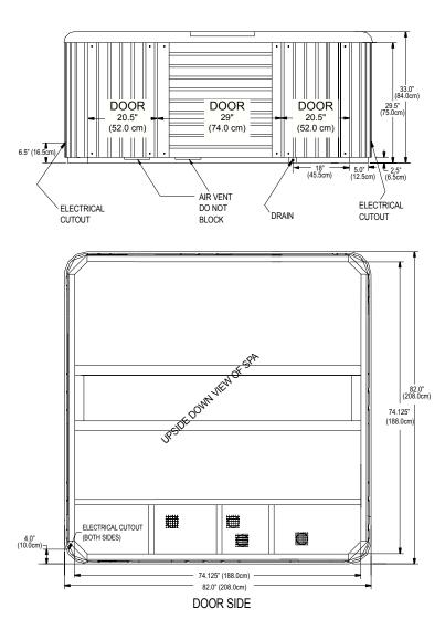
**NOTE: WATKINS WELLNESS** recommends that the **TARINO** be installed on a minimum 4" (10 cm) thick reinforced concrete pad or structurally sound deck able to support the "dead weight" found in the spa specification chart.
