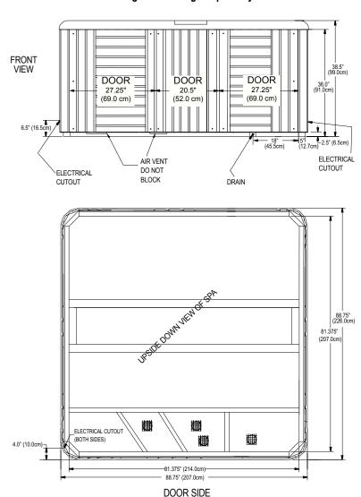
**NOTE: WATKINS WELLNESS** recommends that the **PALATINO** be installed on a minimum 4" (10 cm) thick reinforced concrete pad or structurally sound deck able to support the "dead weight" found in the spa specification chart.
