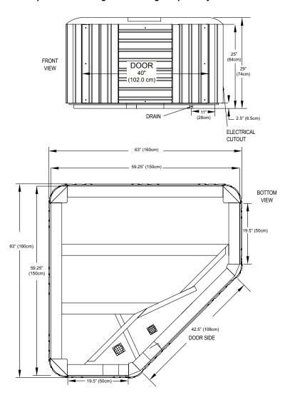
**NOTE: WATKINS WELLNESS** recommends that the **AVENTINE** be installed on a minimum 4" (10 cm) thick reinforced concrete pad or structurally sound deck able to support the "dead weight" found in the spa specification chart.
