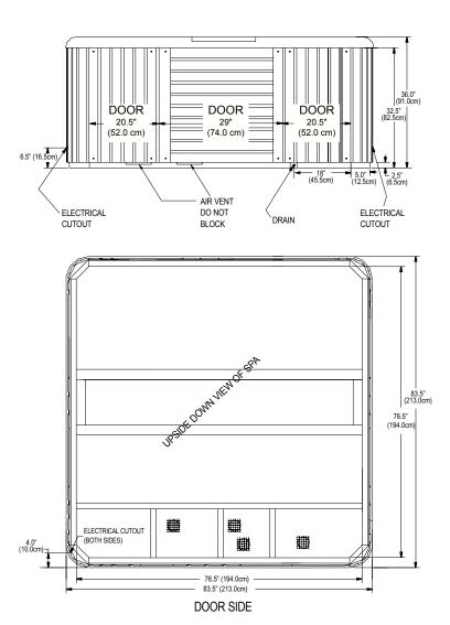
**NOTE: WATKINS WELLNESS** recommends that the **MARINO** & **VANTO** be installed on a minimum 4" (10 cm) thick reinforced concrete pad or structurally sound deck able to support the "dead weight" found in the spa specification chart.
